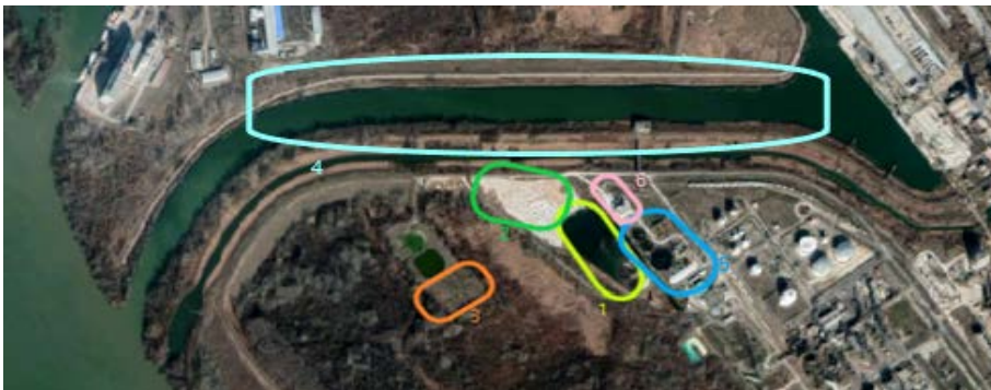
Fig. 1. Location of the waste material in the oil-petrochemical complex: 1. Non-stabilized sludge; 2. Stabilized sludge; 3. Contaminated material from NATO bombing; 4. Wastewater channel; 5. Wastewater treatment plant; 6. Sludge stabilization plant.
