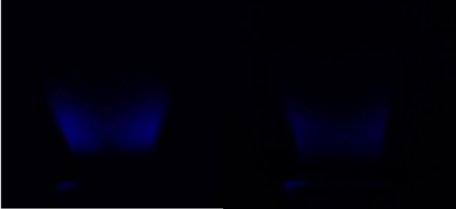
Fig. 4. Images of \text{CH}^* emission of propane (left) and methane (right); air equivalence ratio = 1.20.
